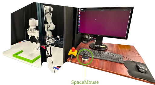
Figure A.5: Real workspace setup for human-in-the-loop data collection. The human operator provides online correction through a 3Dconnexion SpaceMouse while monitoring the robot’s execution.
