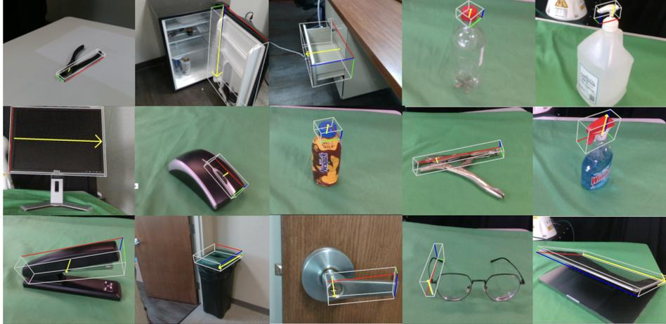
Figure 6: A3VLM predictions on various real-world objects using a single RGB image. A3VLM is able to perform correct inference on challenging real world objects, even for those with transparent or reflecting surfaces.
