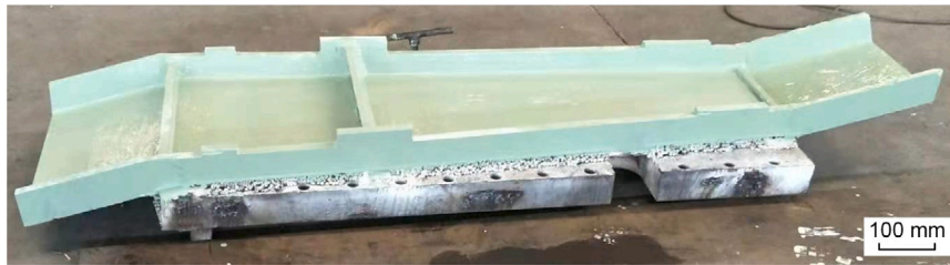
Fig. 16. Pylon beam of civil aircraft fabricated by additive manufacturing. (For interpretation of the references to colour in this figure legend, the reader is referred to the web version of this article.)
