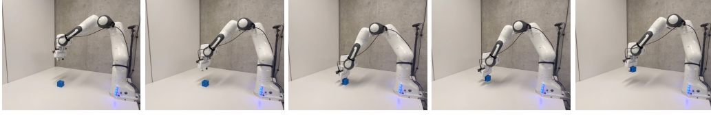
Figure 7: Real-world Deployment: We show an example episode of our policy performing the cube picking task on a Franka robot in the real world.
