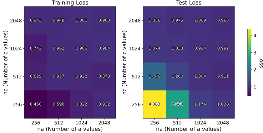
Figure 16: Training (left) and test (right) loss as a function of n_a (number of multipliers a ) and n_c (number of increments c ) for XSLRR-16/8 with 3 control bits.
