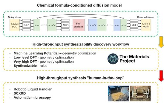
Fig. 1: Overview of the workflow. At the top the architecture of the chemical formula-conditioned diffusion model. In the middle the workflow developed within the Material Project infrastructure.[9] Bottom, high-throughput experimental synthesis.
