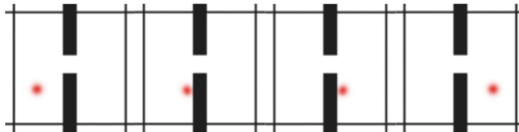
Figure 6: Example of a bad local minima when relaxing the dynamics constraint into a penalty function. The dynamics are nonzero for the middle transition, but both the states and actions are at a local minima; there’s no direction they can move locally to reduce the dynamics loss further.
