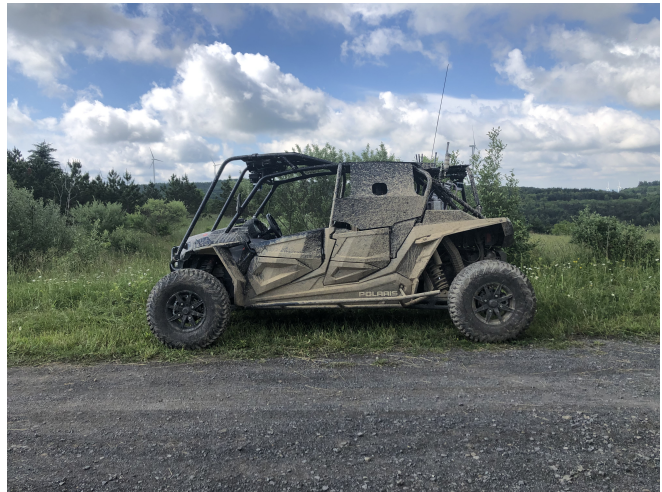
Fig. 1: Polaris RZR: Side by Side outfitted with sensors and computers in a mixed-feature environment. Kinodynamic constraints were determined via human-expert driving to enable the vehicle to autonomously navigate off-road environments at high speeds.
