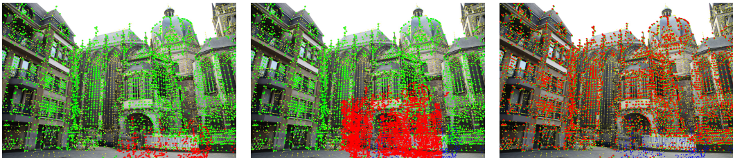
Figure 1: Direct image alignment is a technique for aligning scenes based on image intensities. Recent learning-based methods seek to improve its success rate by increasing the convergence basin. We derive an analytical solution to the core idea of such methods, the Gauss-Newton loss, enabling fine-grained control over the basin of convergence. As a result, we can successfully align two scenes despite a highly imprecise initialization. From left to right, the example above illustrates the convergence of the reprojected keypoints (red) to the ground truth (green) by optimizing the SE(3) camera pose with our analytical solution. The blue color is the re-projection in the first iteration.
