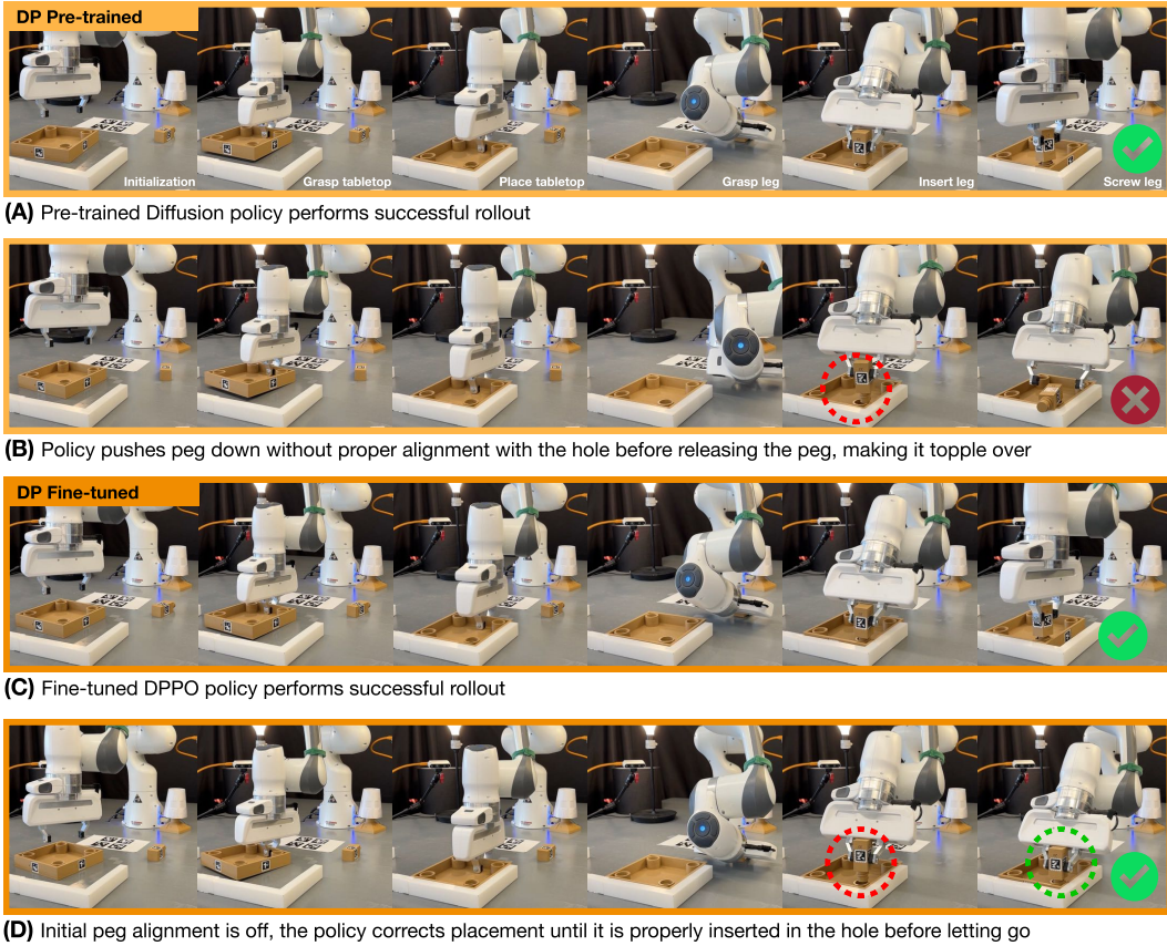
Figure 23: Qualitative comparison of pre-trained vs. fine-tuned DPPO policies in real evaluation. (A) Successful rollout with the pre-trained policy. (B) Failed rollout with the pre-trained policy due to imprecise insertion. (C) Successful rollout with the fine-tuned policy. (D) Successful rollout with the fine-tuned policy that requires corrective behavior.
