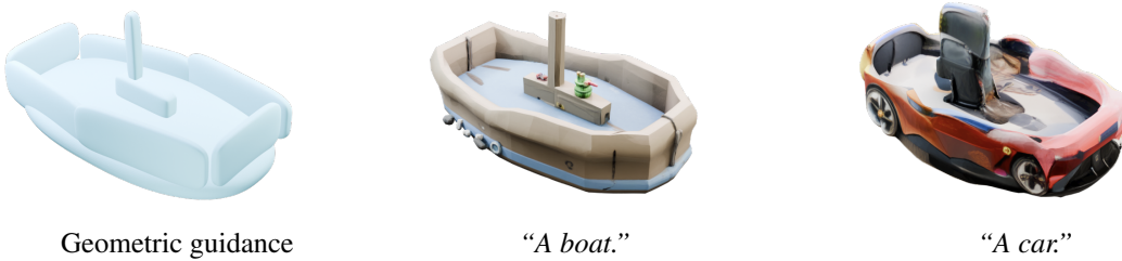
Figure 8: Contrasting conditioning. We use a coarse geometric sketch of a boat ( left ) as geometric control and pair it with two different textual prompts: “A boat.” ( middle ) and “A car.” ( right ). When the prompts align, SpaceControl produces a coherent result. When they conflict, the model injects car-like appearance cues (e.g. wheels) while preserving the underlying boat geometry.
