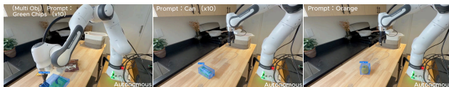
(c) Robotics: Franka Emika Panda autonomously grasping objects specified by open-vocabulary text prompts (“Green Chips”, “Can”, “Orange”).
