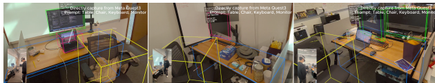
(b) Augmented Reality (Meta Quest 3): passthrough AR with 3D bounding boxes rendered in real time across three desk scenes.
