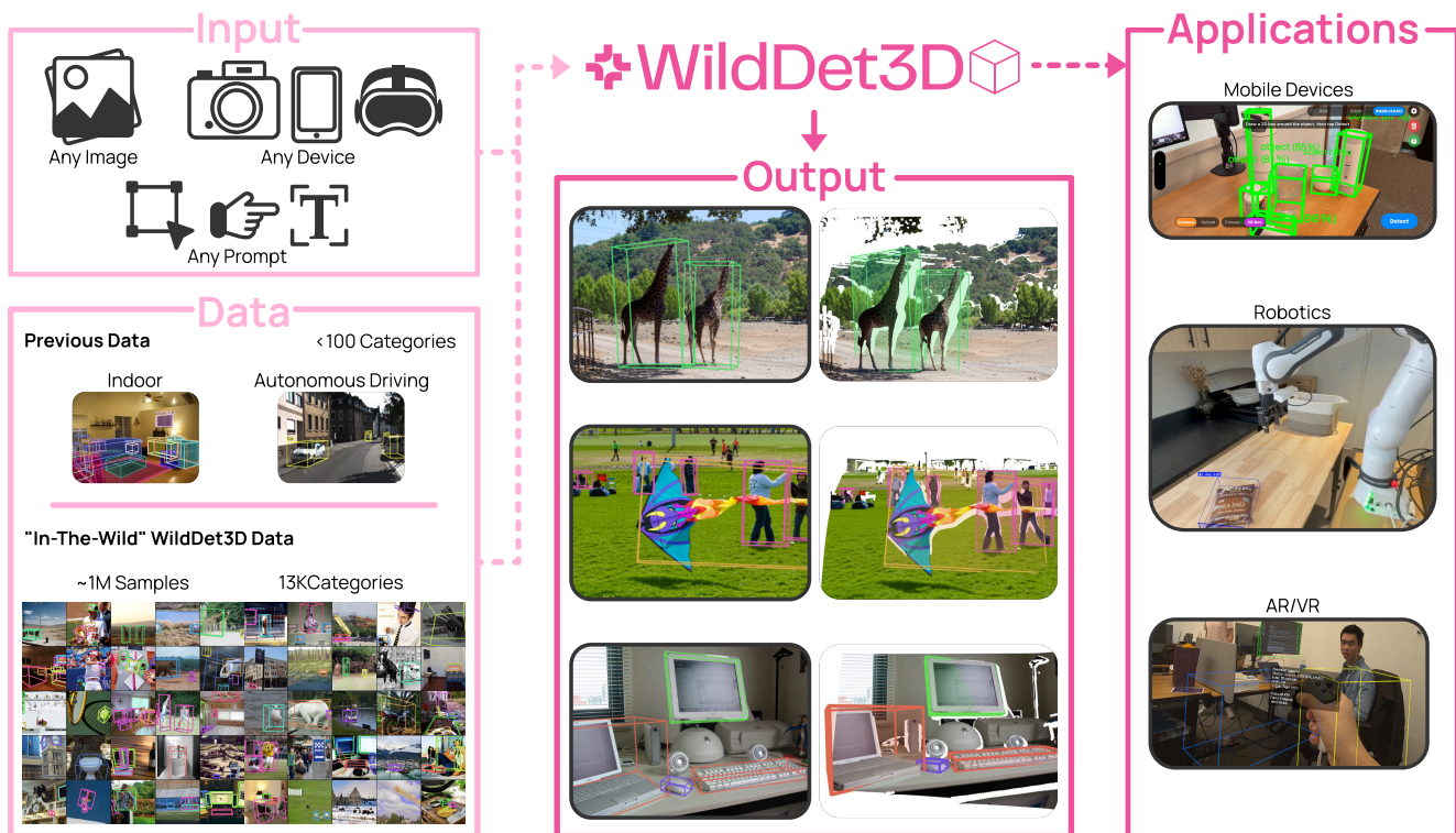
Figure 1. Overview of WildDet3D. Given a single RGB image and an optional depth map, WildDet3D performs open-vocabulary monocular 3D object detection with flexible prompt modalities—text, 2D point clicks, or 2D bounding boxes—and predicts full 3D bounding boxes for the specified objects. The model gracefully leverages additional geometric cues when available. To train WildDet3D for broad generalization, we also curate WildDet3D-Data, a large-scale in-the-wild dataset with approximately 1M human-verified samples spanning 13K categories.
