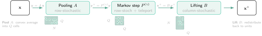
Figure 2: Zoom on the lifted Markov operator ( W_{\text{flow}} ). This panel magnifies the green Flow module from Fig. 1. A reservoir state x \in \mathbb{R}^N is first pooled to coarse cells via a row-stochastic map A \in \mathbb{R}^{Q \times N} (rows sum to 1), yielding y = Ax . Short-horizon dynamics on the coarse graph are applied by P^{(\gamma)} \in \mathbb{R}^{Q \times Q} , a row-stochastic Markov matrix with optional teleport parameter \gamma , giving y^+ = P^{(\gamma)}y . Finally, the signal is lifted back to neurons by a column-stochastic map B \in \mathbb{R}^{N \times Q} (columns sum to 1), producing x^+ = By^+ . Altogether, W_{\text{flow}} = BP^{(\gamma)}A with x^+ = W_{\text{flow}}x , which is the contractive, data-driven component blended into the stable recurrent operator in the main schematic.
