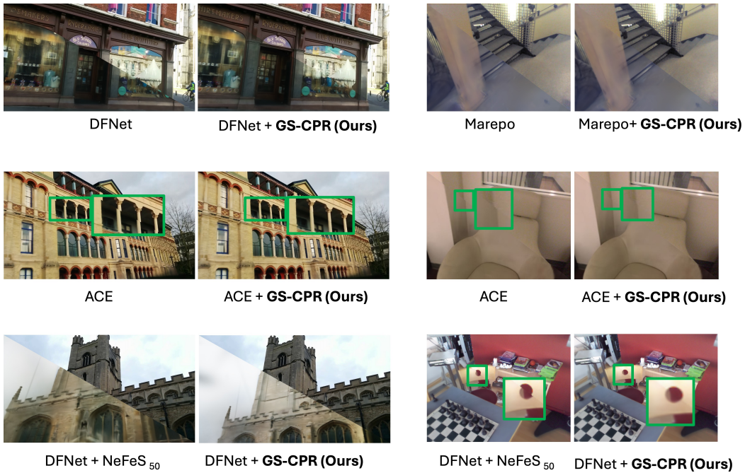
Figure 11: Each subfigure is divided by a diagonal line, with the bottom left part rendered using the estimated/refined pose and the top right part displaying the ground truth image. Patches highlighting visual differences are emphasized with green insets for enhanced visibility.
