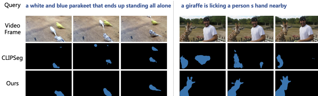
Figure 4: The visualization of segmentation results. Our model is better than CLIPSeg in segmenting unseen categories.
