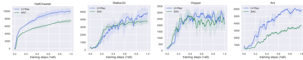
Figure 3: We show the learning curves in Mujoco control compared to SAC. The x -axis shows the training iterations and y -axis shows the performance. All plots are averaged over 4 random seeds. The shaded area shows the standard error.
