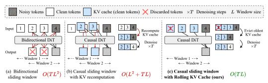
Figure 3: **Efficiency comparisons for video extrapolation.** When performing video extrapolation through sliding window inference, (a) bidirectional diffusion models trained with TF/DF [10, 73] do not support KV cache. (b) Prior causal diffusion models [69, 100] require re-computing KV when shifting the window. (c) Our method does not recompute KV and enables more efficient extrapolation.
