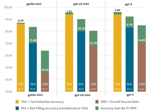
Figure 1: Impact of slot-filling accuracy. Slot filling drives end-to-end success: On the Enterprise Tool-Inventory Dataset (ETID) with complex schemas, we report TSA, SFA, and OSR; green overlays show absolute gains from JTPRO over baselines, highlighting that argument correctness is critical for OSR.
