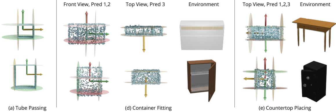
Figure 7. **Geometry Grounding Visualizations.** We plot the learned vectors (as arrows) and planes (as disks) on top of input environment point clouds. We also show the object model next to point clouds for a clearer view of object structure. For (d) Fit, we visualize predictions in two views for clarity. Please refer to Appendix B.1 for more visualizations.
