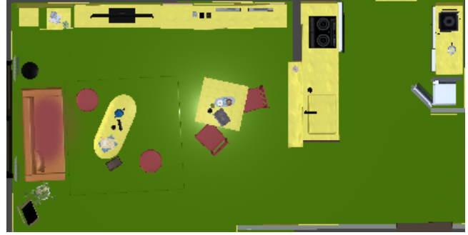
Figure 4: An example of a plane in a scene that represents a supportable posture. Different colors represent supported movements, among which green represents the area where you can stand, red represents the area where you can sit, orange represents the area where you can lie down, and yellow represents the area where you can lean. It should be noted that some components have multiple colors, indicating that they can support multiple postures. e.g. sofa.
