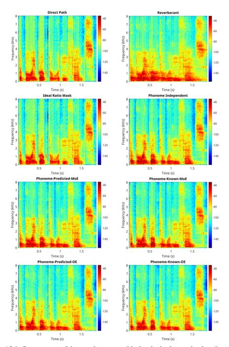
Figure A3.1: Spectrograms of the speech utterance "the boy broke the wooden fence" generated for direct path speech, reverberant speech, enhanced reverberant speech after applying the ideal ratio mask and estimated masks with the phoneme independent model, mixture-of-experts (MoE) model with predicted and known phonemes, and Omni-Expert (OE) model with predicted and known phonemes.
