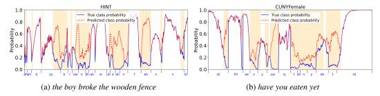
Figure 2: Framewise probabilities of true and predicted phoneme classes of reverberant speech utterances from (a) HINT and (b) CUNY-Female datasets using the GRU+A classifier. True class labels are annotated on the x-axis. Shaded regions indicate incorrect predictions.
