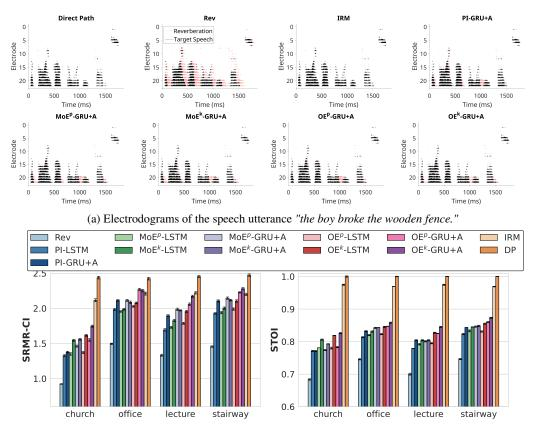
(b) Room-specific estimated marginal means and 95% confidence intervals of speech-to-reverberation modulation energy ratio for cochlear implant users (SRMR-CI) and short-time objective intelligibility (STOI) scores.
