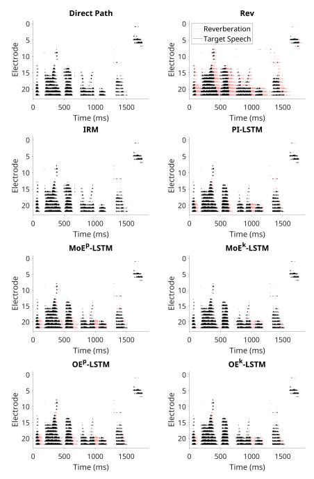
Figure A3.2: Electrodograms of the speech utterance "the boy broke the wooden fence" generated for direct path speech, reverberant speech (Rev), enhanced reverberant speech after applying the ideal ratio mask (IRM) and estimated masks with the phoneme independent model (PI), mixture-of-experts model with predicted and known phonemes ( $MoE^{p/k}$ ), and Omni-Expert model with predicted and known phonemes ( $OE^{p/k}$ ).
