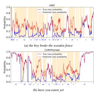
Figure A5.2.1: Framewise probabilities of true and predicted phoneme classes of reverberant speech utterances from (a) HINT and (b) CUNYFemale datasets using the long short-term memory (LSTM) classifier. True class labels are annotated on the x-axis. Shaded regions indicate incorrect predictions.
