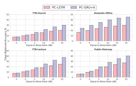
Figure A8.3.1: Phoneme classifier (PC) performance in noisy reverberant room conditions using the long short-term memory (LSTM) model and the gated recurrent unit + attention (GRU+A) architecture. TTB, two-talker babble.
