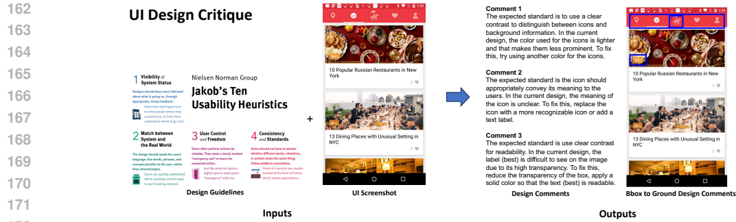
Figure 1: Illustration of the UI Design Critique Task, which takes in a UI screenshot and a set of design guidelines and outputs a list of design comments with corresponding bounding boxes (Bbox).
