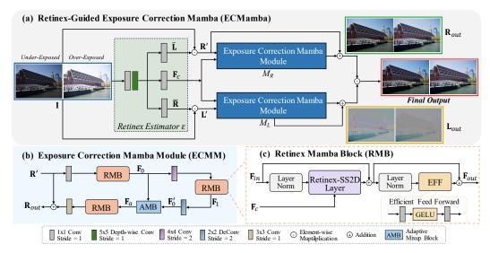
Figure 2: The overall architecture of our proposed Retinex-based framework for exposure correction, which includes a Retinex estimator  $\mathcal{E}$  and primary restoration network  $\mathcal{M}_R$  and  $\mathcal{M}_L$ .
