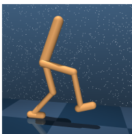
Figure 23: Walker(18, 6, 24) : This domain includes a planar walker. This environment simulates a simple locomotion task of humans, with the agent possessing two legs and advancing in an upright posture. It comprises three distinct tasks, and our experiment focus the walk task. In this task, the objective is to control the walker to maintain an upright torso posture, achieve the specified torso height, and maintain a consistent forward velocity.
