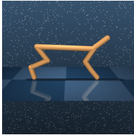
Figure 21: Cheetah(18, 6, 17) : This domain features a planar bipedal and it is able to crawl forward by its two legs. It involves a single task, namely the run task. In the initial state of the environment, the agent's pose is random, typically in a non-standing position. In this task, the challenge is to control the planar biped to achieve an upright standing position and subsequently propel it forward into a running motion with a targeted forward velocity.
