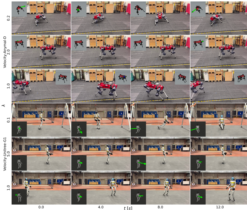
Figure 5: MOPO-PPO policy deployment on ANYmal D and Unitree G1 under varying levels of model-uncertainty penalization. The green arrow indicates the commanded velocity target. With appropriate uncertainty penalization, the robots explore novel behaviors in imagination while staying within reliable regions of the learned model, resulting in high-performance policies comparable to state-of-the-art sim-to-real methods.
