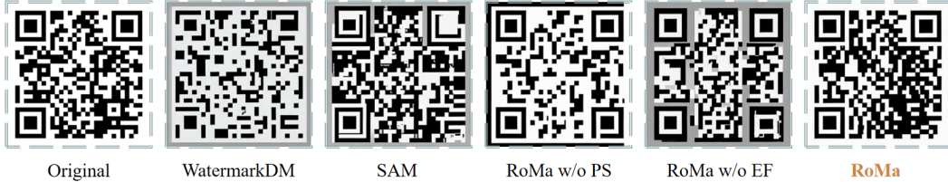
Figure 4: Visual comparison of watermark preservation capabilities across different watermarking schemes after 6,000 fine-tuning steps on MS-COCO-2017. Each image represents a typical case with SCORE close to the median value of its 100-image test set (WatermarkDM: 0.550, SAM: 0.509, RoMa w/o PS: 0.578, RoMa w/o EF: 0.594, RoMa: 0.750 ). The leftmost image shows the original watermark for reference.
