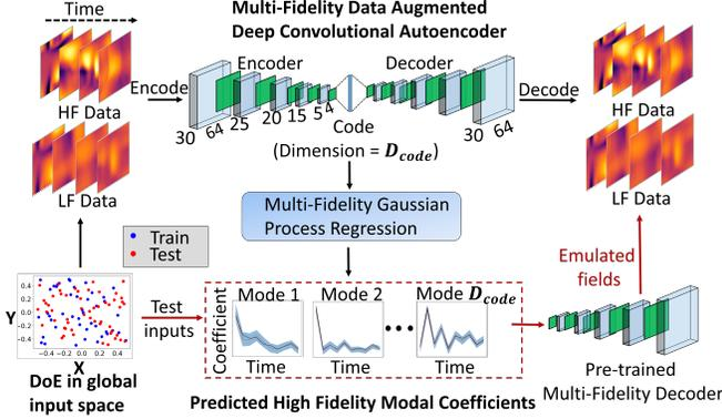
Figure 1: Schematic overview of the proposed multi-fidelity spatio-temporal modeling framework (MF-STM).
