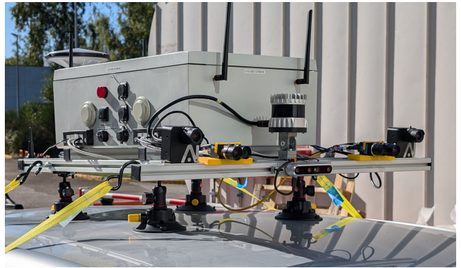
Fig. 1. Real prototype of our data-acquisition system. The sensor suite comprises dual RGB and dual event cameras, a LiDAR, and an IMU. An Arduino-based timing unit and a GPS-RTK receiver are mounted inside the enclosure for hardware-level synchronization.
