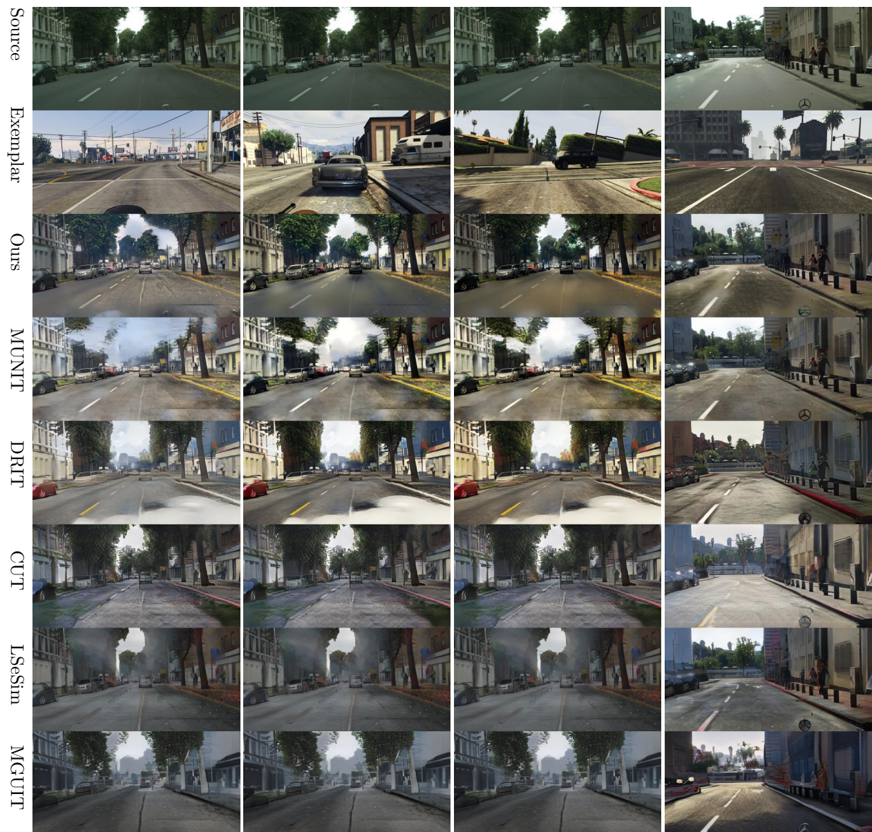
Figure 16: Qualitative comparison with other methods. CS \rightarrow GTA. Our method yields a high output diversity, yet preserves the trees in the first, second, and third columns. The road has the closest appearance to the exemplar with our method in the last column.
