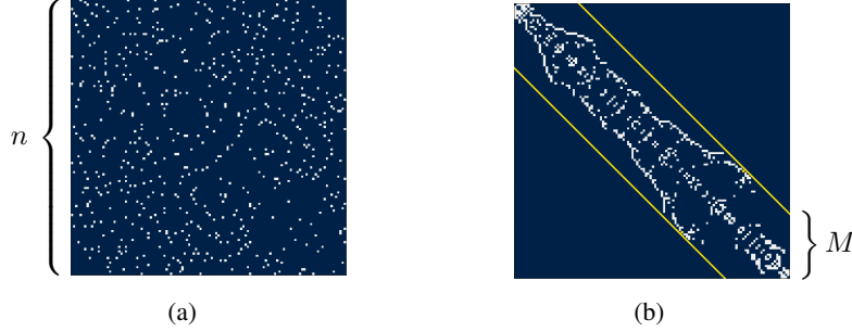
Figure 2: (a) Shows the adjacency matrix of a random graph under a random node ordering. (b) Depicts the adjacency matrix of the same graph under a BFS ordering. We can see that the entries are closer to the diagonal under the BFS ordering, allowing us to represent the upper triangle using smaller slices of length M .
