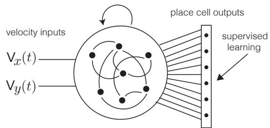
Figure 2. The setup of the path integration task: A single layer recurrent neural network with 4096 hidden units receives two-dimensional velocity inputs and is trained in a supervised manner to output (an encoding of) the two-dimensional position.
