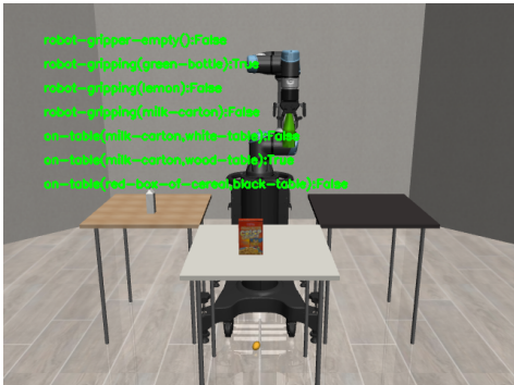
(d) State estimation using threshold=0.2 and Factored State Sampling. Features which cannot co-exist cancel each other by comparing probabilities, a list of canceled, canceler pairs follows: [(‘robot-gripper-empty()’, ‘robot-gripping(green-bottle)’), (‘robot-gripping(milk-carton)’, ‘robot-gripping(green-bottle)’), (‘on-table(milk-carton,white-table)’, ‘on-table(milk-carton,wood-table)’), (‘robot-gripping(milk-carton)’, ‘on-table(milk-carton,wood-table)’)].
