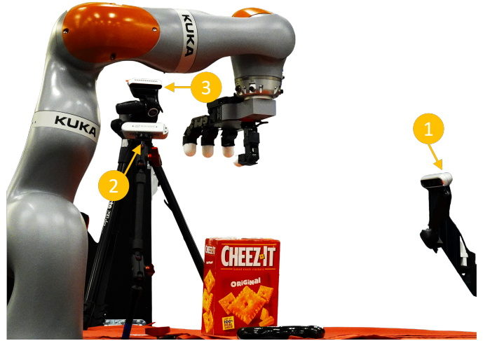
Fig. 5: Real robot setup showing the Kuka iiwa arm equipped with a left Allegro hand and the configuration of the three RGB-D cameras.
