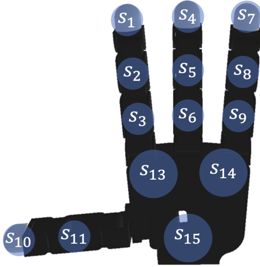
Fig. 16: Placement of collision spheres for computing collision loss, each sphere has radius of 0.015
