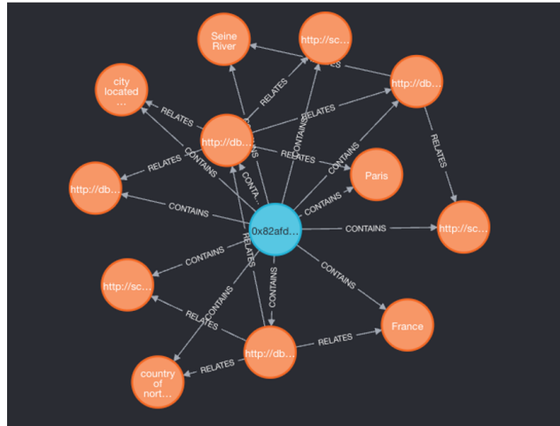
Figure 5. Example subgraph from a knowledge graph: This subgraph was generated in response to the input prompt, ‘Can you tell me about the capital of France?’ AI agents produced answers from which triplets were extracted. These triplets are then ingested into the graph, with each node and relationship being categorised into a node or relationship group corresponding to the AI agent operator’s identifier. The light blue node represents the identifier (i.e., public address) of the AI agent operator. The ‘CONTAINS’ relationship denotes ownership, while the ‘RELATES’ relationship captures predicate information as its value type.
