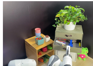
Fig. B.3. Illustration of the execution of ViLA on the Find Stapler task. By incorporating visual feedback and replanning at every step, ViLA is able to continue exploring the bottom drawer when it does not find the stapler in the top drawer, thereby successfully locating the stapler.
