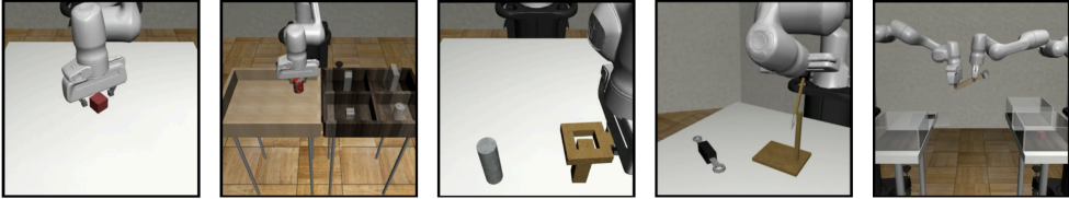
Figure 4: Robomimic tasks: lift, can, square, tool-hang, transport. Among these tasks, square features multi-modal behavior, tool-hang requires high-precision manipulation, transport is particularly challenging because its long-horizon complex multi-modal nature.
