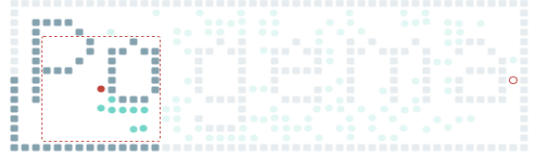
Figure 2: Partial observation with FOV. Agents (red dots) observe information within their FOV (red frame). Gray dots represent obstacles (dark) and other agents (light). Image cited from 2 .
