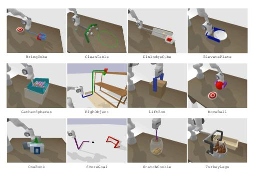
Figure 3: VLMGINEER produces innovative tool designs and their corresponding actions across 12 diverse tasks in ROBOTOOLBENCH that are challenging to perform using a general-purpose robot arm and gripper.
