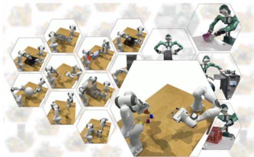
Figure 1: Selected bimanual tasks from the benchmark as well as real-world examples. Due to the architecture design the method can easily be transferred to other robots as the policy outputs a 6-D pose and is agnostic to the underlying controller.
