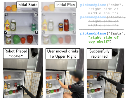
Figure 6: APRICOT Adapts to Changes in Environments. The user’s preference requires drinks to be placed together. After the user disrupts the scene and moves the drinks to the right side of the top shelf, APRICOT’s closed-loop planner is able to adjust its plan and properly satisfy the user’s preference in the newly changed environments.
