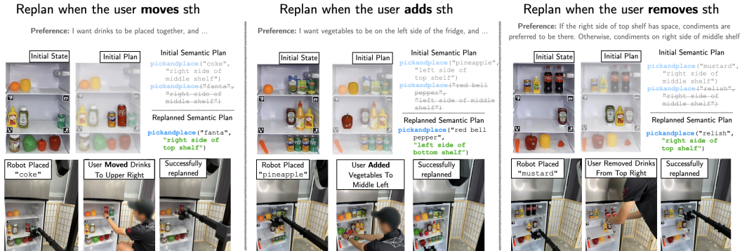
Figure 10: Examples of how APRICOT’s task planner can replan and handle different ways a user could affect and change the environment.
