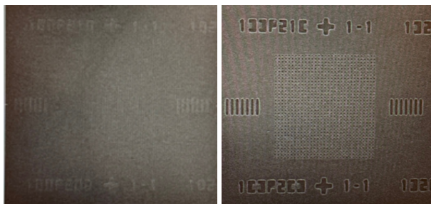
Figure 3. Qualitative lithography comparison. Left: commercial n-Butyl Acetate baseline. Right: representative formulation generated by LithographyAgent. The example illustrates improved qualitative pattern definition under the tested conditions. This comparison is intended as proof-of-concept evidence rather than a comprehensive experimental benchmark.
