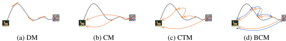
Figure 1: An illustrative comparison of score-based diffusion models, consistency models, consistency trajectory models, and our proposed bidirectional consistency models. (a) DM estimates the score function at a given time step; (b) CM enforces self-consistency that different points on the same trajectory map to the same initial points; (c) CTM strengthens this principle of consistency, which maps a point at time t back to another point at time u \leq t along the same trajectory. (d) BCM is designed to map any two points on the same trajectory to each other, removing any restrictions on the mapping direction. When the mapping direction aligns with the diffusion direction, the model adds noise to an input image. Conversely, if the mapping direction is opposite, the model performs denoising. This approach unifies generation and inversion tasks into a single, cohesive framework.
