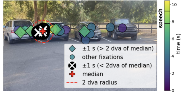
Figure 4: Temporal-spatial filtering of eye gaze data. Fixations colored by time. Black lines on the color bar mark speech onset and end. Diamonds represent fixations within \pm 1s of speech onset; all others are circles. Any diamond within 2 dva of the diamonds’ median (red +) is spatially filtered and rendered as white crosses on black circles and passed onto IRIS.
