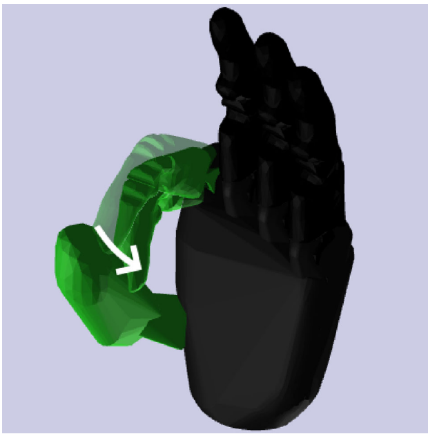
Fig. 16 Example for how the joint angles were biased for hand calibration. Bias effect is exaggerated for clarity. (Color figure online)
