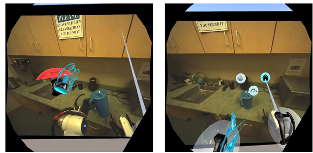
Fig. 7 (Left) View from the operator’s perspective. A force-feedback sphere (described in Sect. 6.2) in red shows the operator the force on AVATRINA’s left hand. The blue ghost hand shows the sensed configuration of the operator’s left hand. (Right) Heads-up display menu enables semi-autonomous functionalities: texture-sensing mode (left), arm “homing” (right), and base speed adjustment (center) icons. (Color figure online)
