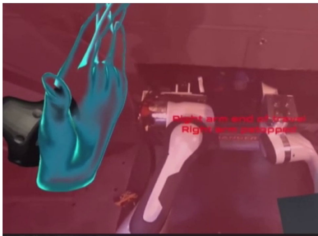
Fig. 25 The operator's view after AVATRINA's right arm engaged mechanical brakes in response to excessive force. [Best viewed in color.]
