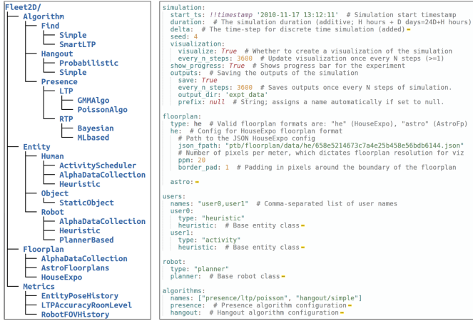
Fig. 4. (left) The hierarchical code structure of the scenario components in Fleet2D. It is extensible, and new functionality continues to be integrated continually. (right) The configuration file offers a high-level interface to define this scenario (details folded to conserve space). It mirrors the code components for ease of use and development.
