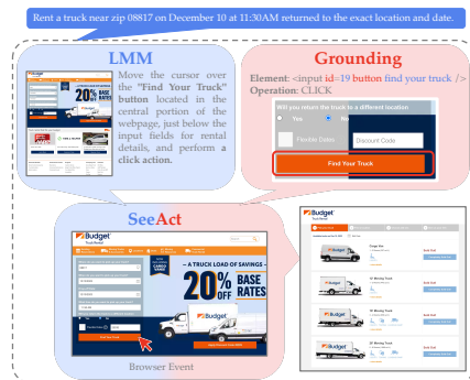
Figure 1: SEEACT leverages an LMM like GPT-4V to visually perceive websites and generate plans in textual forms. The textual plans are then grounded onto the HTML elements and operations to act on the website.
