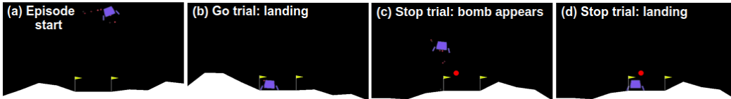
Figure 3: LunarLanderContinuous-v2 with Bomb. (a) Episode starts with the lander placed randomly on top of the frame around the center. (b) Go trial: refers to an episode without a bomb, and it is exactly as the original environment. (c) Stop trial: refers to episodes in which a bomb randomly appears close to the landing pad (between the two flags). (d) It shows a successful landing during a stop trial after avoiding hitting the bomb. By default, the bomb appears in 50% of the episodes.
