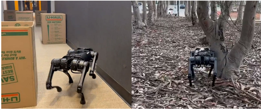
Figure 9: Some failure cases of vision-guided whole-body controller due to limitation of agility. The left figure shows that when walking through a narrow path, the robot can not quickly turn around and collide into the wall. The right figure denotes that it may collide to the tree in the wild, due to the shape of the obstacles are out of the training distribution and the robot can’t adjust quickly enough to avoid.
