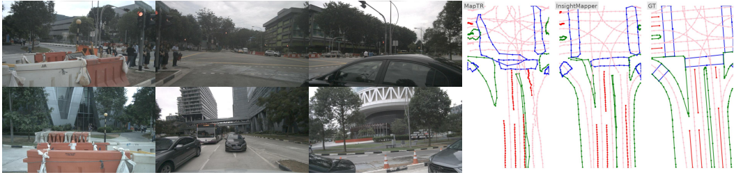
Figure 7: Qualitative visualization. The predicted map contains four classes, i.e., road boundaries (green), lane splits (red), pedestrian crossing (blue), and lane centerlines (pink).
