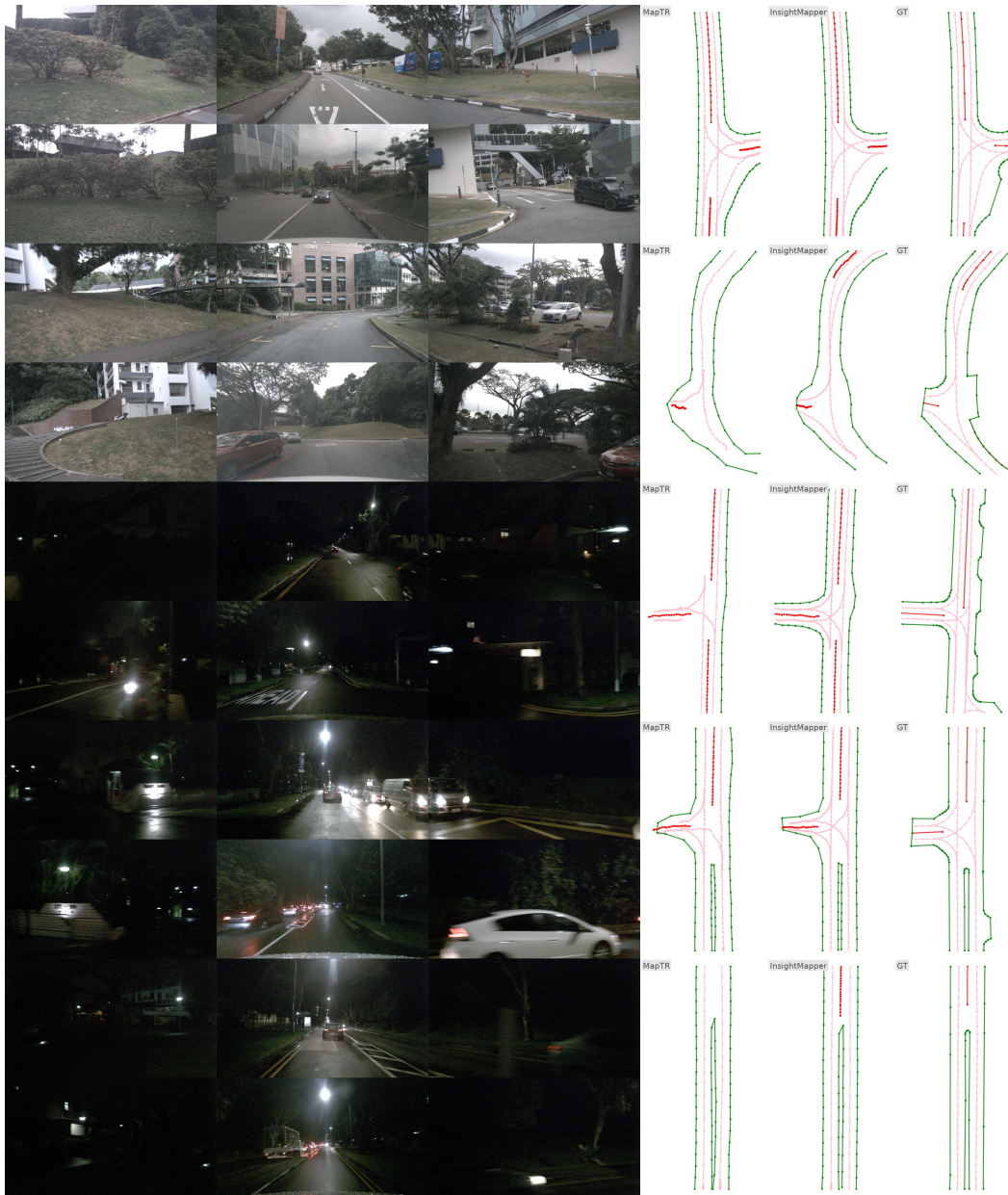
Figure 14: Qualitative visualization. Left three columns are input 6 RGB camera images. For map columns, the first column presents MapTR’s results, the second column features InsightMapper’s outcomes, and the final column depicts the ground truth map. The predicted map contains four classes, i.e., road boundaries (green), lane splits (red), pedestrian crossing (blue), and lane centerlines (pink).
