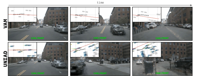
Figure 3. Driving behavior comparison on NeuroNCAP [28]. UniAD [22] and VaVAM are evaluated in a frontal collision scenario. Images: frontal camera. Inset plots: top view of scene evolution, with objects (gray boxes) and guiding path (red line) highlighted for visualization only. While UniAD detects and forecasts the oncoming vehicle (blue), it fails to react. VaVAM successfully deviates to avoid collision and safely returns to its lane, without explicit supervision.
